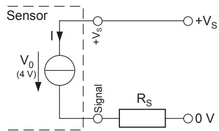
When using the current output, the resistor to be connected must not exceed a specific value:
