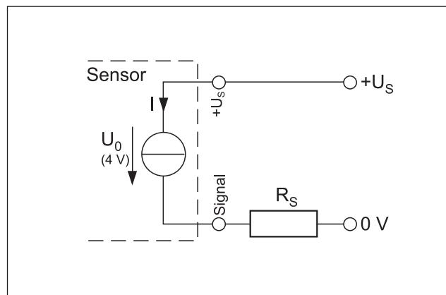
When using the current output, the resistor to be connected must not exceed a specific value:
