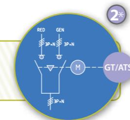
Available from 200 up to 3150A depending on configurations, Telergon offers a wide range of Enclosed Transfer Switches for changing Mains-Alternative (Gen Set), or similar applications both manual and automatic.
